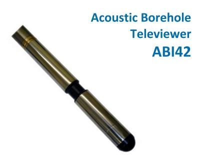
The digital **Acoustic Borehole Televiewer ABI42** outputs a continuous power ultrasonic wave train emitted by a rotating transducer for scanning the sidewall of the borehole thus providing an oriented, continuous 360° image of this one. The sonde can be run into a borehole filled with either mud or water.
