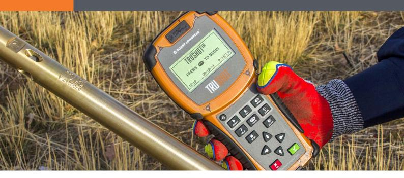
TruShot™ is an accurate magnetic survey tool optimized for driller deployment. Made for durability, precision and simplicity, drillers can capture high-quality 3D hole path data with confidence.
