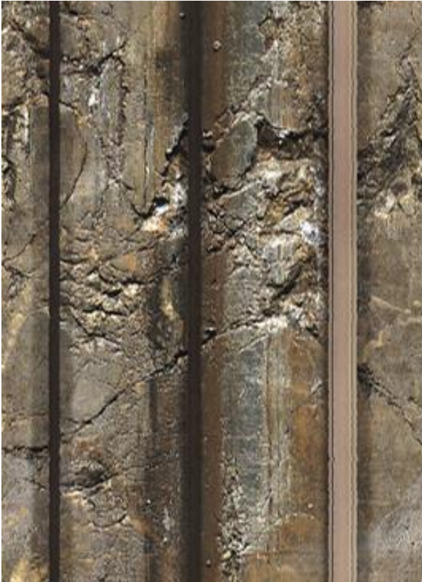
Example OTV image section acquired using the hazardous hole deployment system in a 200m dry up-hole. Longitudinal artifacts are from the carrier arms which extend past the imaging head.
